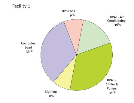
Figure 1: Comparison of actual benchmarking data from two data centers showing breakdown of total electricity use per watt of server. Facility 2 uses less than half as much power on infrastructure.
