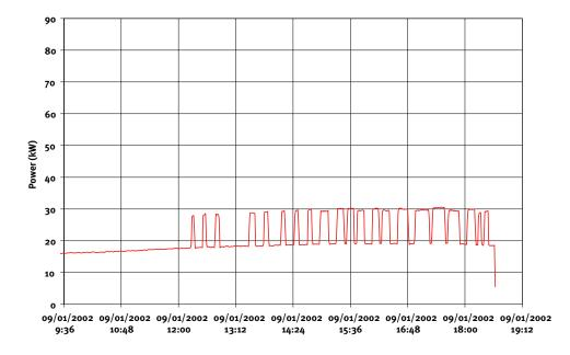
Figure 9: Facility A data center 1 Chiller 1 power
