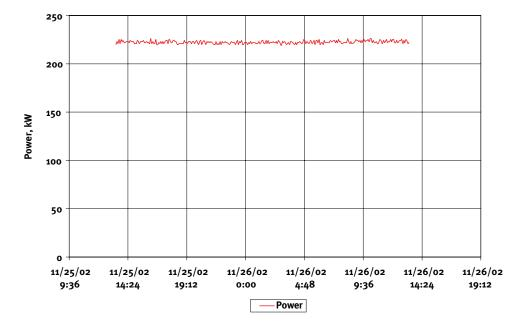
Figure 8: Sample whole-facility data center load variation over 24 hours
