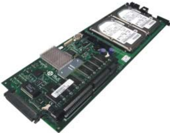
Figure 15 Typical Blade server Source: RLX Technologies
