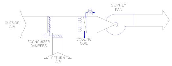
Figure 6. Schematic drawing of a typical air-side economizer.
