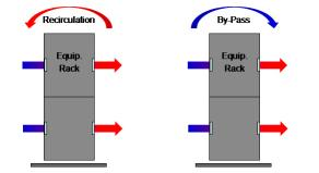
Figure 1. End view of rows showing undesirable recirculation and by-pass air around IT racks.
