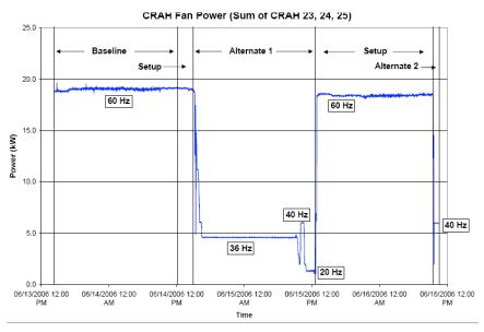
Figure 4. Case study of savings using Variable-Speed Drives on fans ("Alternate 1").
