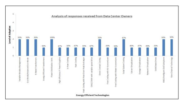
In the electrical system, prioritization has been given to high efficiency IT power supplies followed by energy efficient transformers. 66.7% participants selected Level 1 for IT power supplies and 50% of participants selected Level 1 for transformers. For
