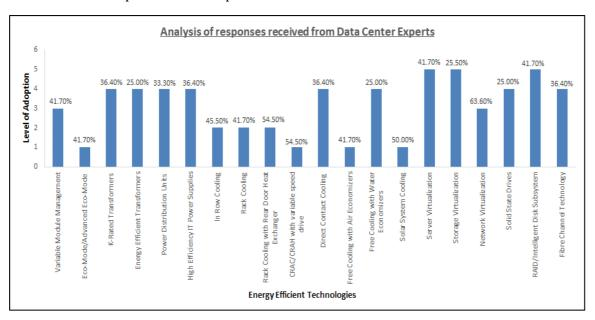
In the electrical Section, prioritization is given to K-rated transformers and high efficiency IT power supplies followed by PDU and energy efficient transformers, signifying a high level of adoption in data centers Level 4 was selected for K-rated Transformers and high efficiency IT power supplies by 36.40% of participants. 33% selected level 4 for PDU and 25% selected Level 4 for energy efficient transformers, still indicating a high level of adoption.
