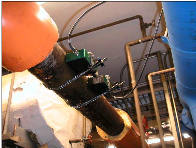
Figure 8. Measurement of Chilled Water Flow
