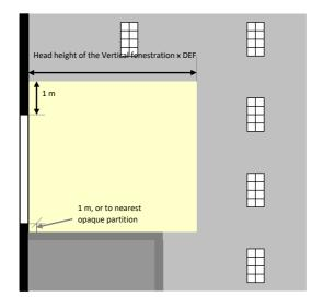
**Daylight Extension Factor (DEF):** factor to manually calculate the daylight area on floor plates. It is to be multiplied by the head height of windows. It is dependent on orientation and glazing VLT, shading devices adjacent to it and building location.
