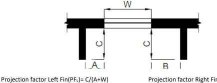
**Projection Factor, overhang and side fin:** average of ratio projection factor for overhang only and projection factor of side fin only.
