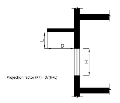
Projection factor, side fin: It is the ratio of the horizontal depth of the external shading projection to the distance from the window jamb to the farthest point of the external shading projection, in consistent units.
