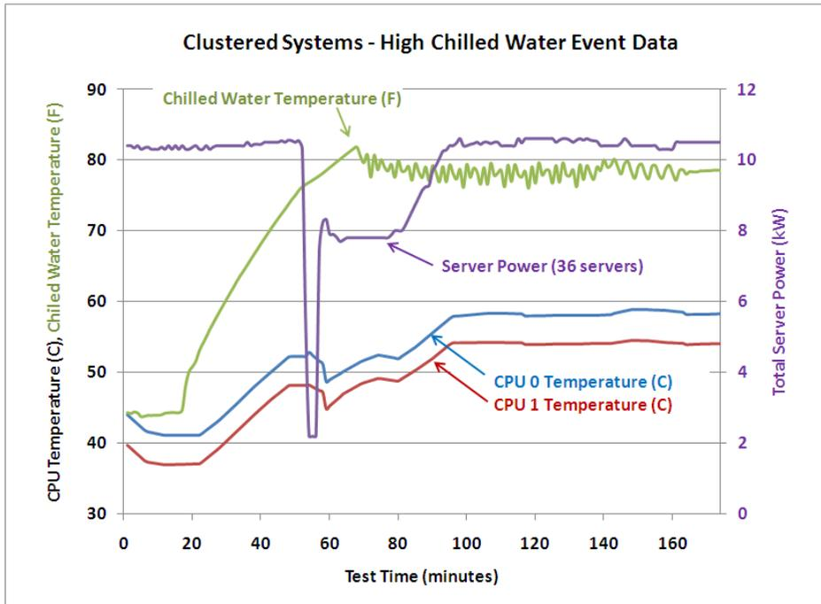
**Figure 3-13: Clustered System Performance During the Facility Event, Resulting in Very High Chilled Water Being Supplied**
