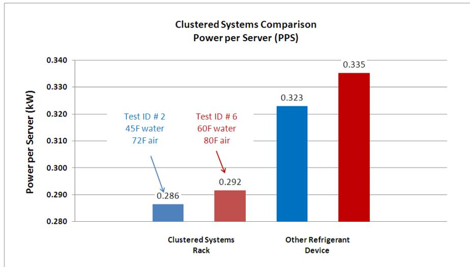
Figure 3-10: Clustered Systems Server Power Comparison
