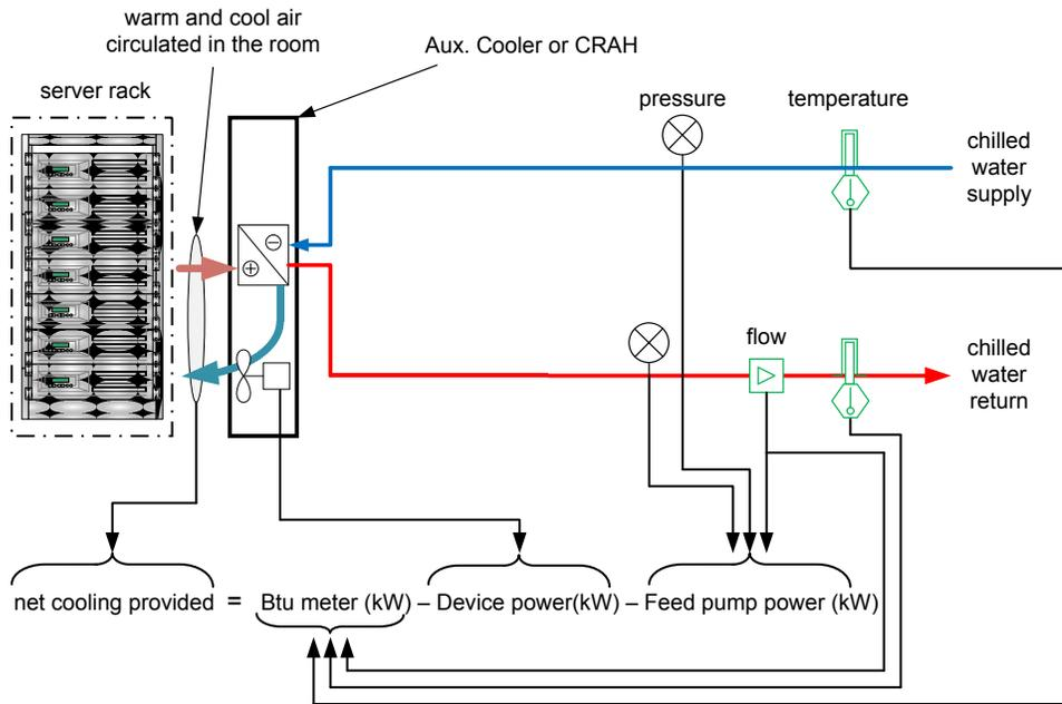
**Figure 2-8: Net Cooling Provided ( $NC_b$ ) – Water Only Cooling
