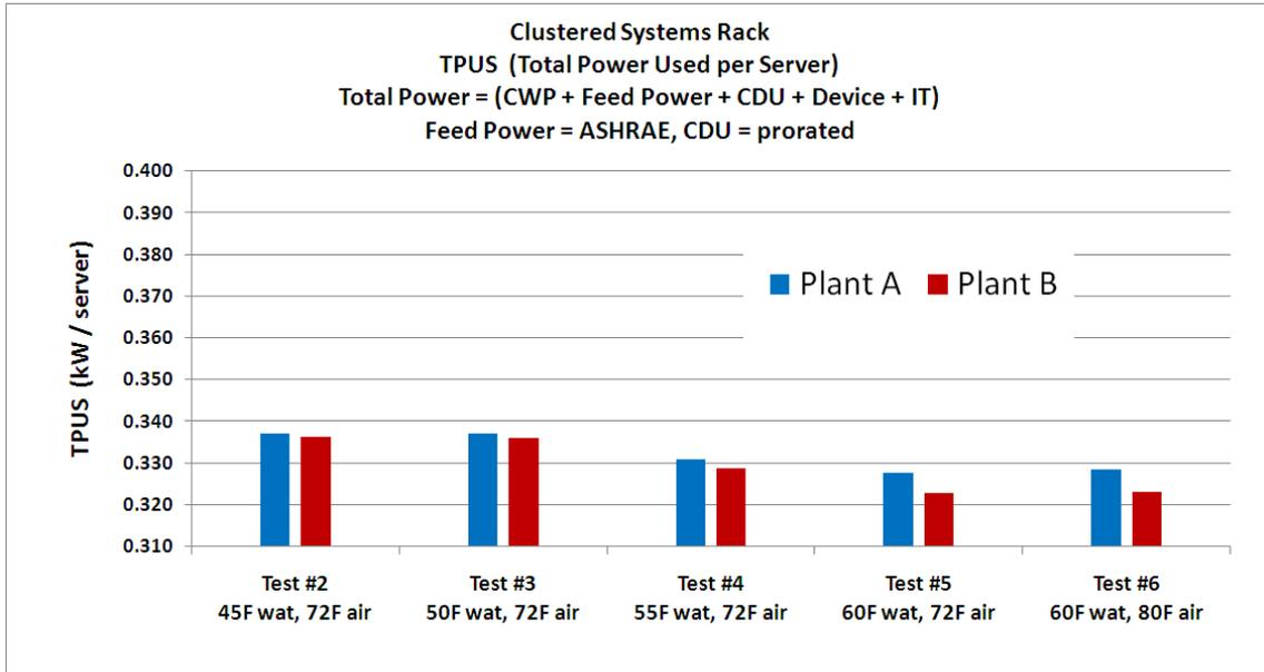
**Figure 3-11: Clustered Systems TPUS Performance using Two Chilled Water Plant Models**
