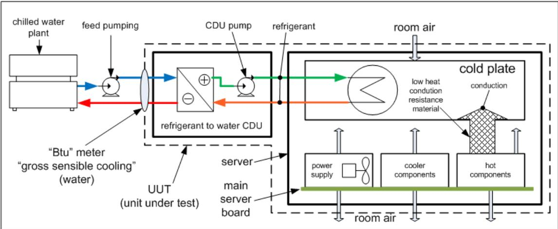
Figure 1-1: Thermal Schematic for the Clustered Systems Design
