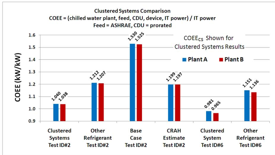
**Figure 3-8: COEE Metric Comparison**
