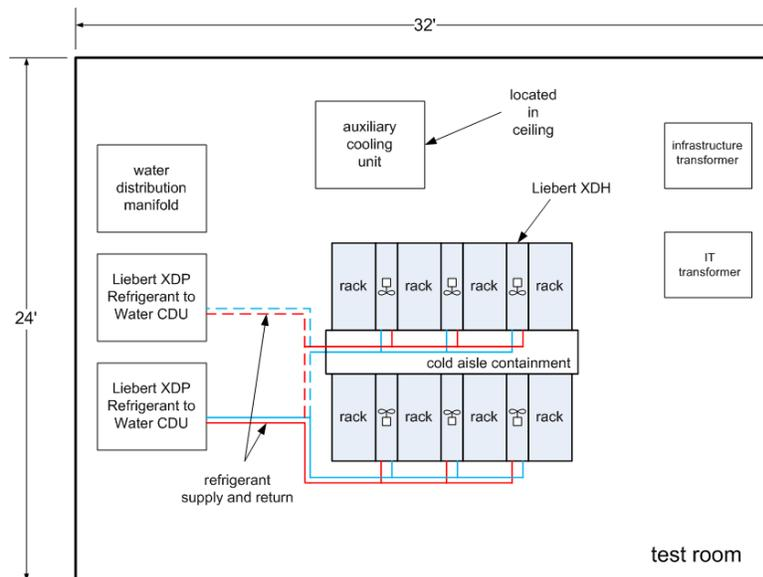
**Figure 2-2: Room Layout for the Other Refrigerant Design Test**
