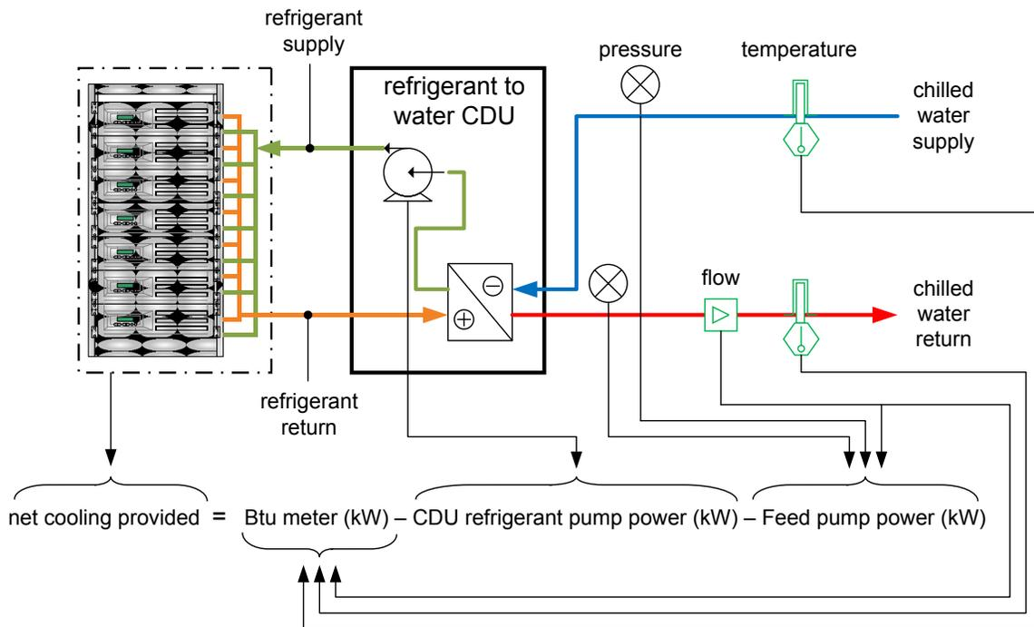
**Figure 2-10: Net Cooling Provided( $NC_b$ ) – Direct Touch Cooling**
