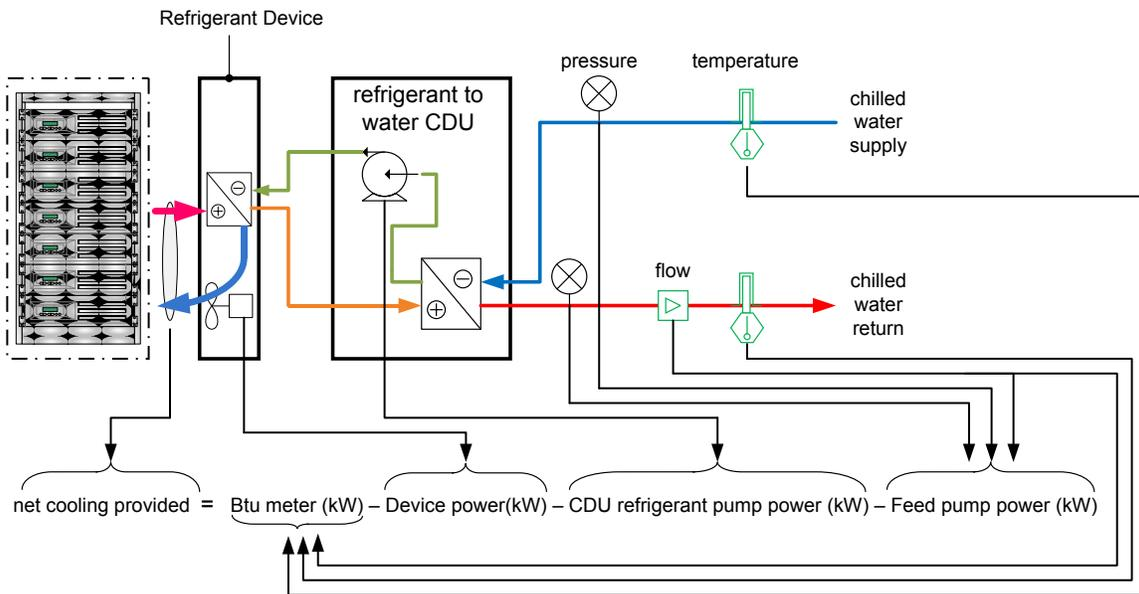
**Figure 2-9: Net Cooling Provided ( $NC_b$ ) – Refrigerant-to-Water Cooling
