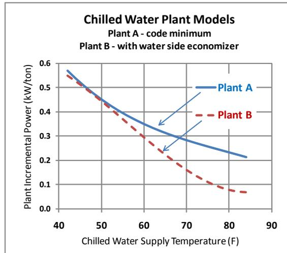
**Figure 2-7: Chilled Water Plant Models (A and B) Electrical Power – Not Including Chilled Water Distribution Pumping Power**
