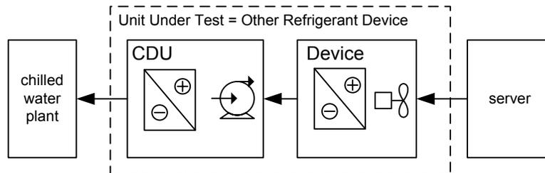
Figure 2-4: UUT Definition Diagram for the Liebert XDH/XDV
