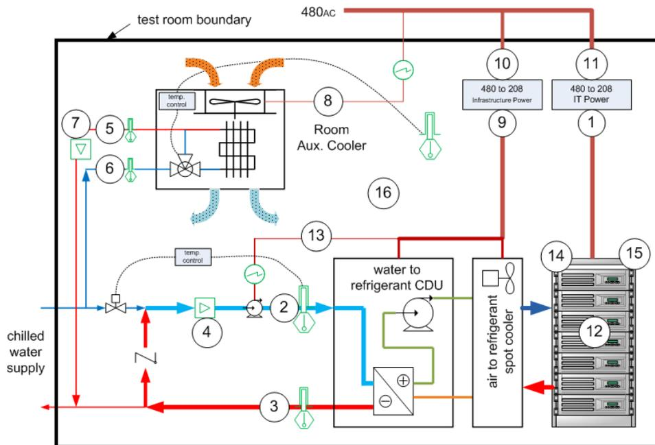
**Figure 2-6: Schematic Locations of the Data Points**
