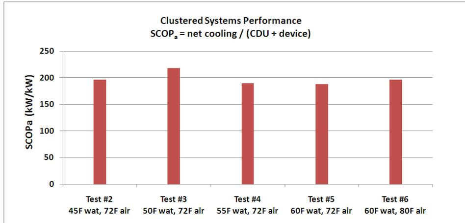
**Figure 3-1: Clustered Systems SCOP<sub>a</sub> Performance**
