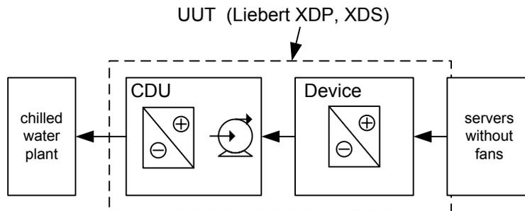
Figure 2-3: UUT Definition Diagram for the Liebert XDP, XDS
