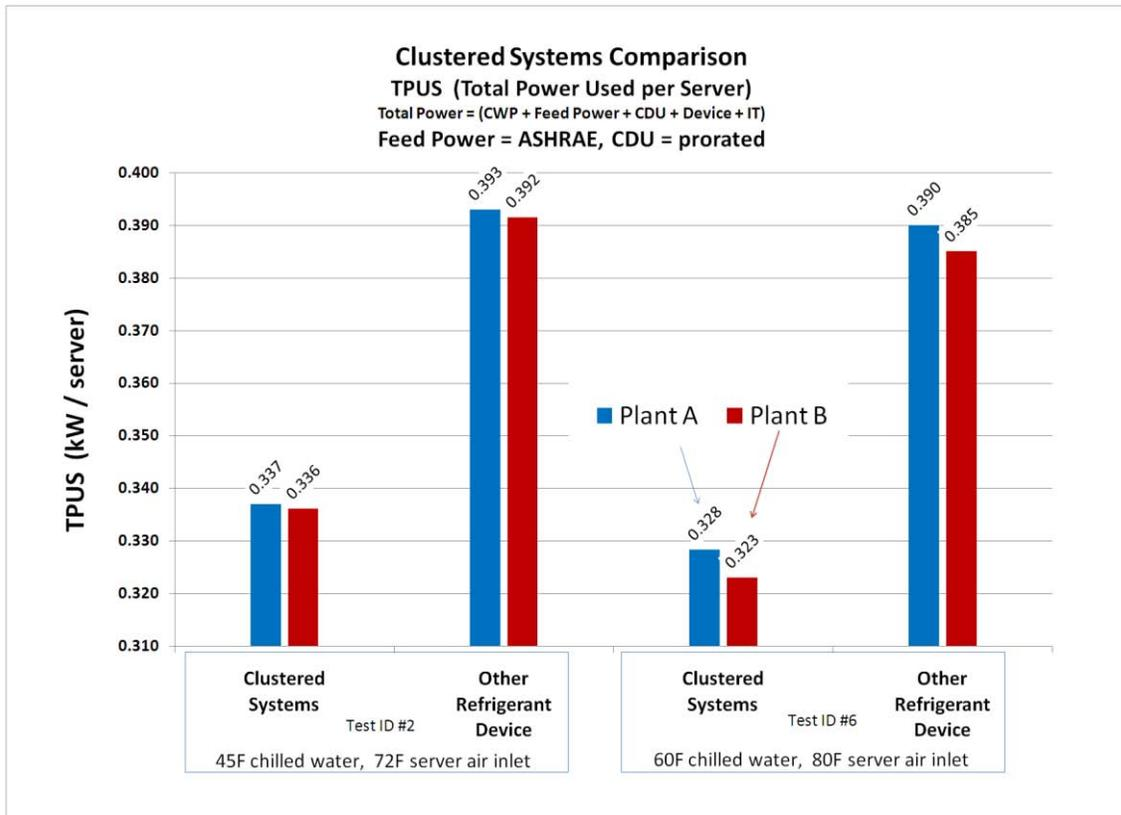
**Figure 3-12: Clustered Systems Compared to Other Refrigerant (Liebert XDH/XDV) for Test 2 and Test 6, for Two Chilled Water Plant Models**
