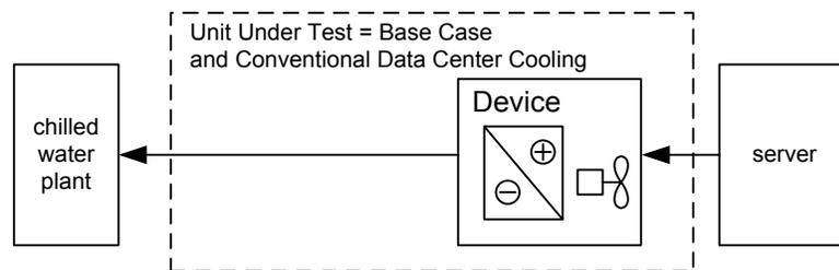
Figure 2-5: UUT Definition Diagram for the Base Case and CRAH Designs
