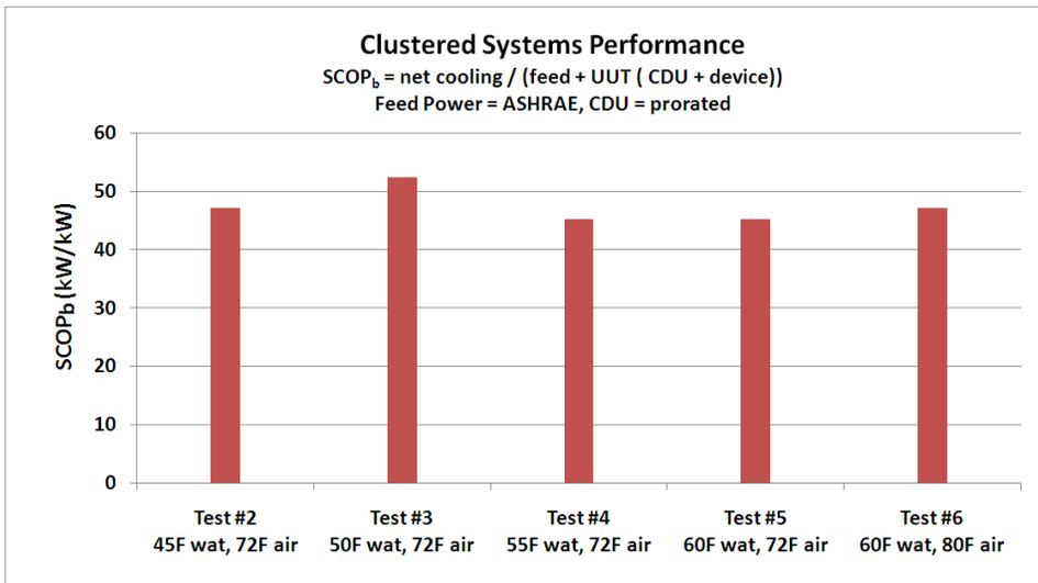
Figure 3-3: Clustered Systems SCOP<sub>b</sub> Performance
