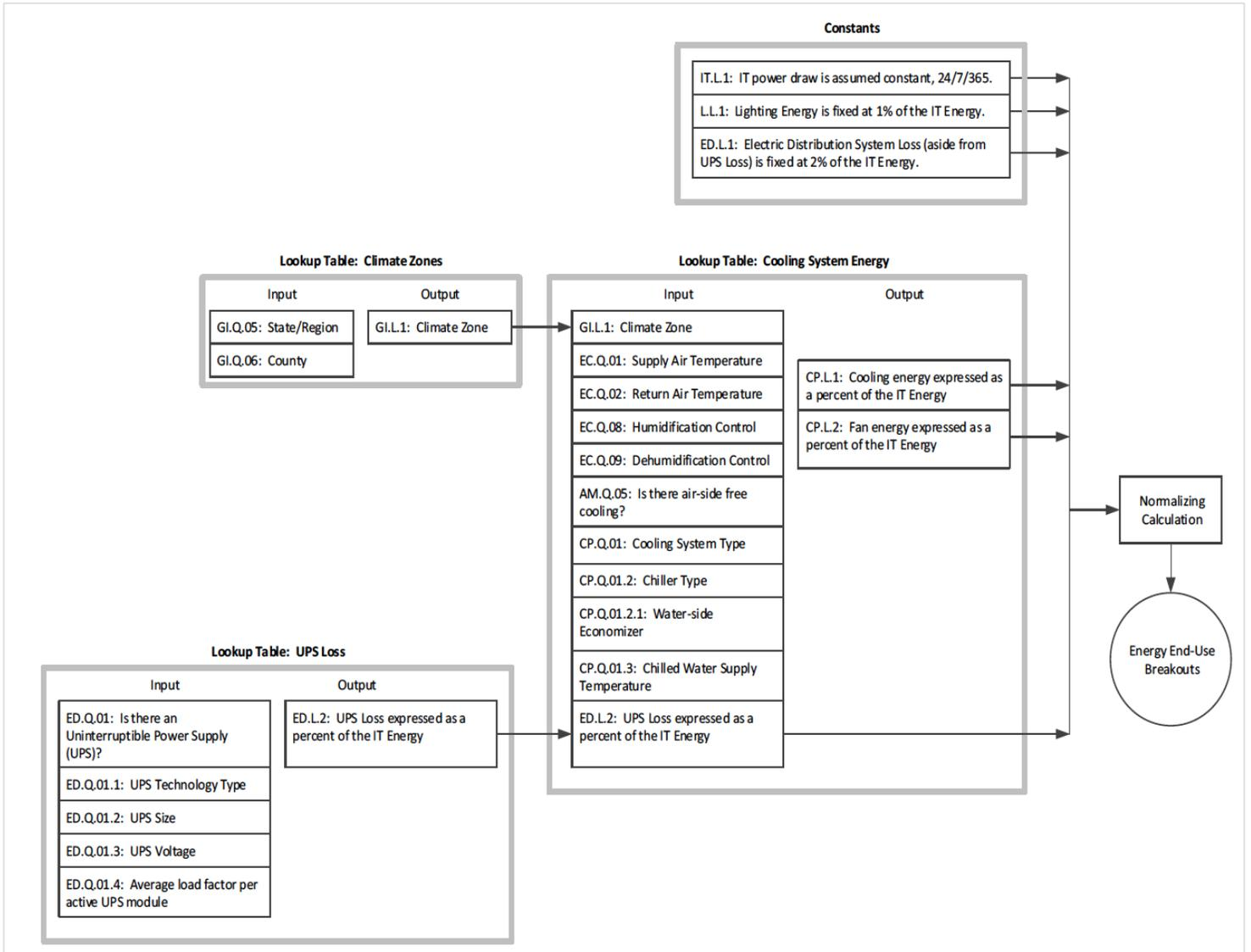
Figure 20: PUE Calculation Method Flow Chart
