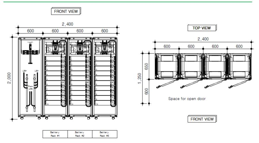
Sample battery solution layout for a 250 kW x 15 m energy storage solution using Lithium ion based technologies
