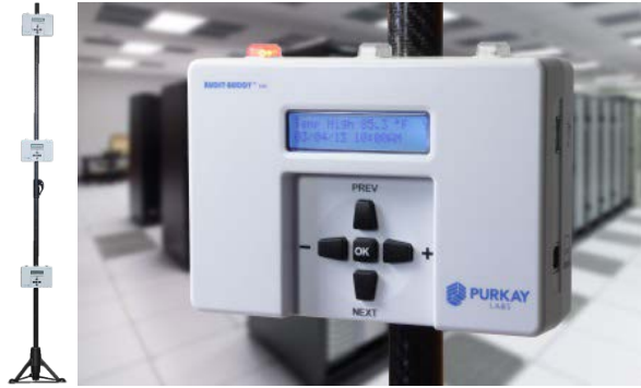
Figure 14: PurkayLabs: Three temperature/humidity (TH1) units mounted on a carbon fiber rod (detail to right, not to scale)
