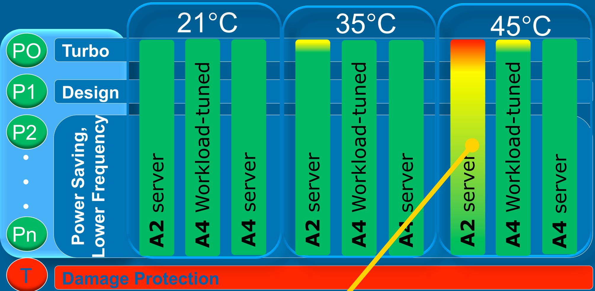
*Unpredictable performance, memory follows a similar trend although throttling mechanism is different*
