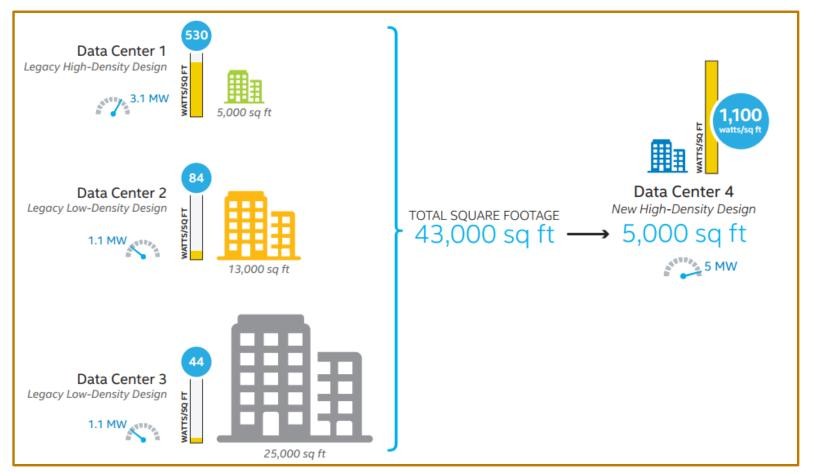
Our high-density design allows for an increase in watts per square foot. Economies of density work similar to Moore's Law: the cost per kW goes down as more kW are put into each square foot of production area.
