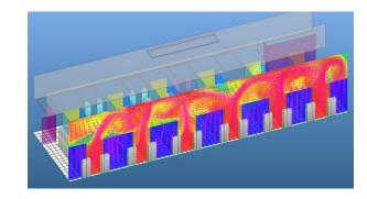
Alternating hot aisles (exhaust air) and cold aisles (supply air) provide efficient air segregation and the exhaust-air plenum allows hot air to easily exit the building.
