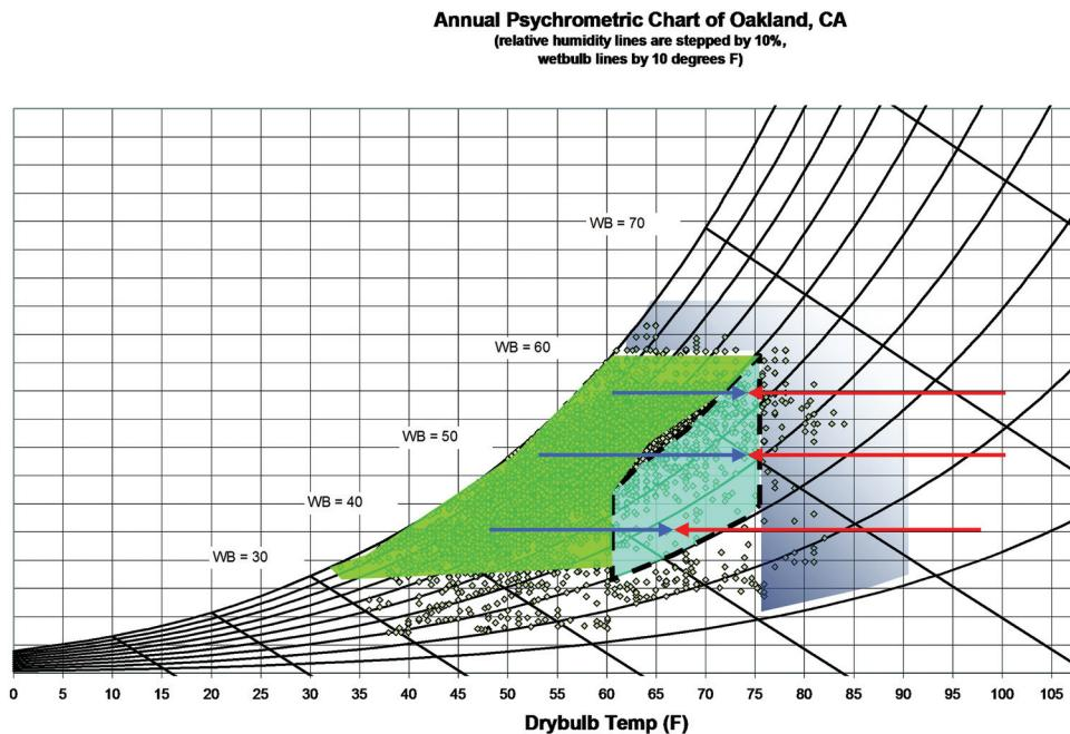
**Figure 5** Psychrometric data for Oakland (adjacent to Berkeley). The dashed line of 60–77°F (16–25°C) dry-bulb and 30–60% RH is the designed supply air condition. The arrows represent mixing of outside air and return air.
