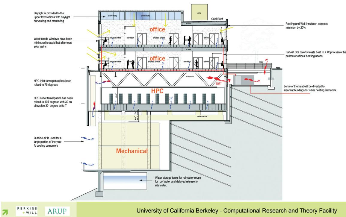
**Figure 2** Building section showing AHU located below computer floor, exhaust air path (return is to left and down to AHUs), and office floors above.
