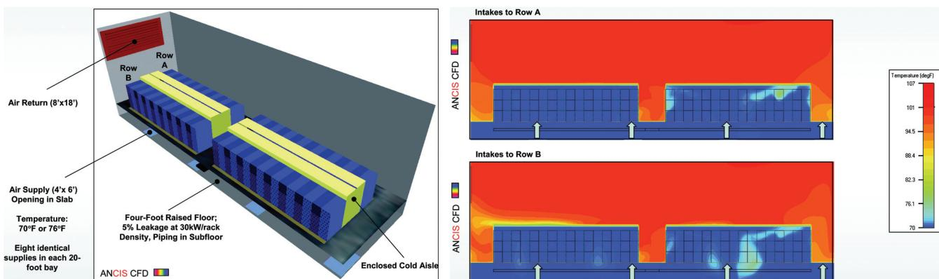
**Figure 8** Computational Fluid Dynamics study was performed to optimize under floor plenum design. [Source: ANCIS Incorporated]
