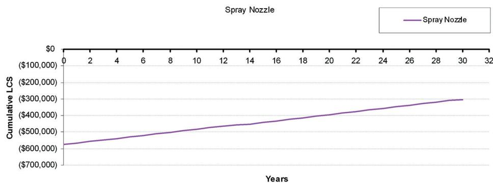
**Figure 6** Life Cycle Cost performance of 'spray nozzle-type' system compared to base-case pad-media type direct evaporative cooler.
