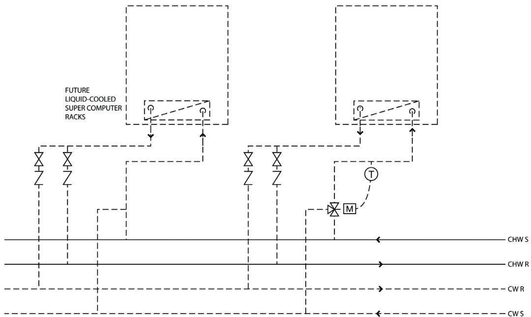
**Figure 4** Four-pipe cooling water system. The chilled water supply and return are the solid lines; the dashed lines are future closed-loop cooling water supply and return (via cooling towers and heat exchangers; see Figure 7).
