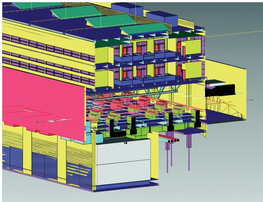
**Figure 3** 3-D image illustrating air movement from outside air louvers through to underfloor plenum via multiple 3'×8' (0.9 m × 2.4 m) punctures at the structural slab. Design documents were produced using 3-D Revit models for better coordination between disciplines. [Source: Arup]
