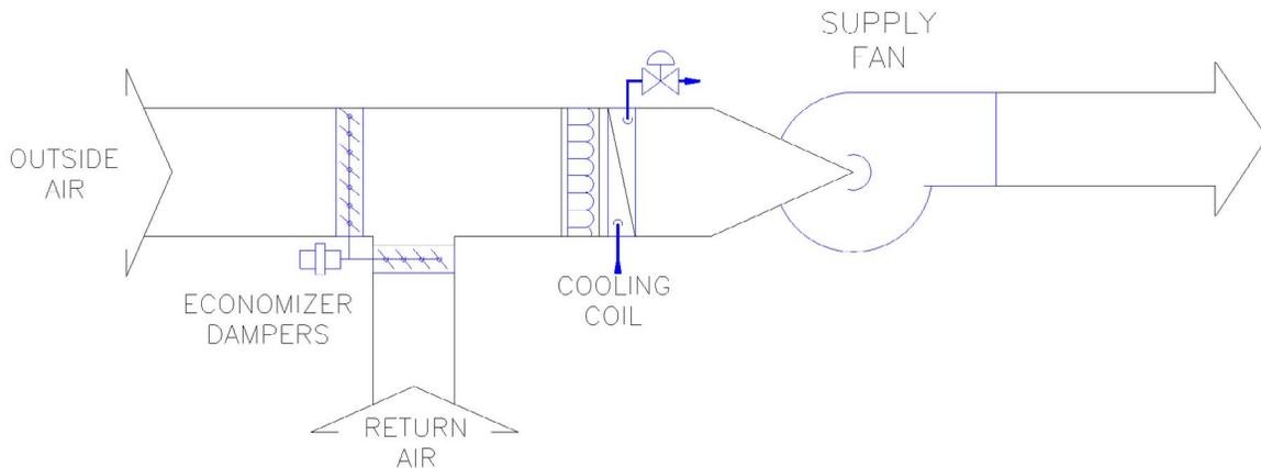
Figure 6. Schematic drawing of a typical air-side economizer.
