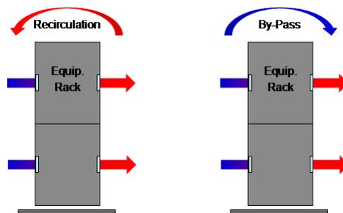
Figure 1. End view of rows showing undesirable recirculation and by-pass air around IT racks.
